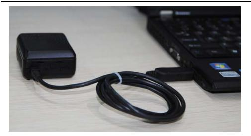
Run MEITRACK Manager.exe , turn on the device and connect it to the computer via USB, the software will automatically indentify the port number and read out all parameter as follow:
