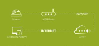
Adopting the high-performance processor and Linux operating system, Meitrack independently develops a new-generation wireless vehicle video surveillance system that uses H.264 video compression/decompression, GPS positioning and wireless data transmission technologies. It is specially designed for mobile video surveillance for different types of vehicles, such as buses, long-distance coaches, taxis, logistics vehicles, armored cars, private cars, etc.
