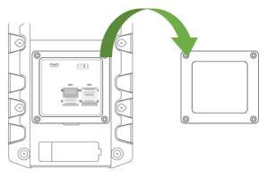
Insert a SIM card into one of the card slots (SIM1: right; SIM2: left).
