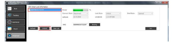
Note: The binding and unbinding functions are only available for the K211G with a LoRa module.
