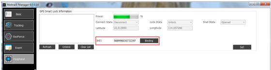
Note: To establish LoRa communication between the K211G and the T399G, the two devices must be bound each other. Please connect the T399G to the computer, and then repeat the above operations to bind the K211G.
