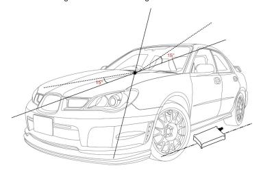
The default harsh acceleration and braking alert values are 230 mG and -300 mG respectively.
