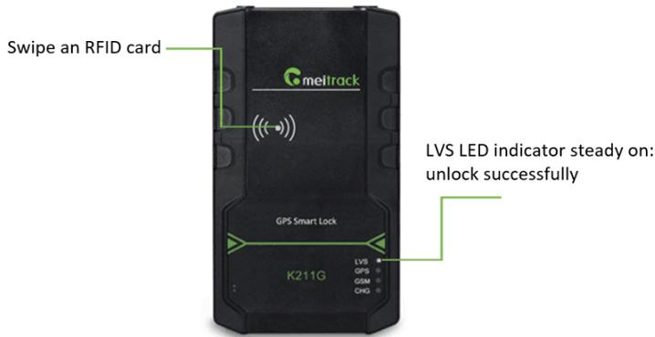
Note: In the locking or unlocking state, if you swipe an unauthorized RFID card, the buzzer will beep twice. If you swipe an authorized RFID card, the buzzer will beep once. After the K211G is unlocked, if you do not pull out the lock rope within one minute, the K211G will be locked automatically.
