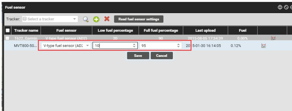
Note: When the fuel detection port of the MVT600/T1/MVT800/T333 is connected to the fuel level sensor, no formula is required on MS03. When the sensor detects that the fuel is lower than the lower limit or is higher than the upper limit, an alarm will be generated.
