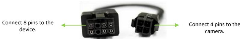
Note: To connect the camera to T1/T333, a 4 pin to 8 pin conversion cable is required.
